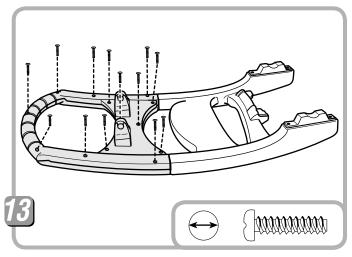
• Insert 13 - #8 x ¾" screws into the handle top and tighten.
